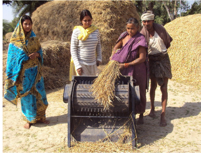
Use of pedal operated paddy thresher
